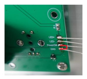
Short the pins connected by the red line in the picture with metal. If everything is normal, the OLED should show the following. (no A\_1350385 are connected to A\_1345897.)
