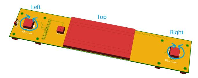
Test to the left and right encoders are working properly. Rotate them as shown by the blue arrows in the diagram, to make sure that the OLED display switches correctly.
